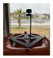
The wind sensor can last 150 hours without being charged. The charging starts when the Calypso is put upside-down on its wireless charge pad (to be placed with labels on the bottom part) and a small red light on the platform becomes blue.
